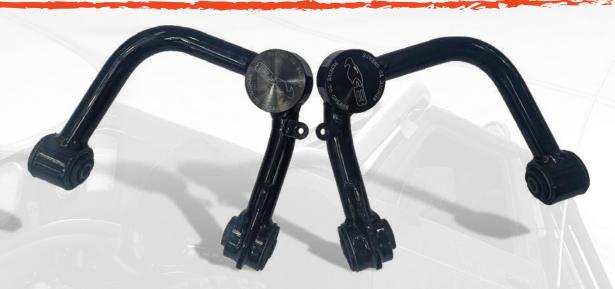
The Blackhawk 4x4 UCA for the N70/N80 with lifts of 25-100mm would be one of the best-known aftermarket UCAs on the market when it comes to fixing the impact on steering kinematics that a lift kit induces. Its design is to be better than original equipment producing more caster than the factory figure. Providing a much better driving experience and steering feel.
