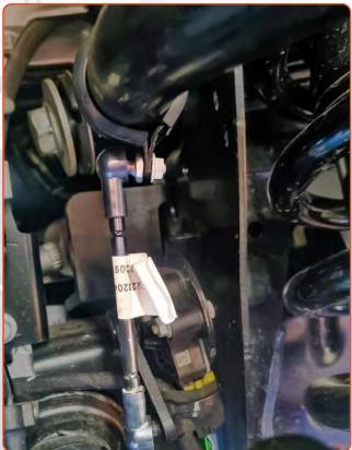
As a temporary solution the following is required to adapt Matrix headlights to the Blackhawk UCA's. Production after batch code J23 will not require this method and will utilise OEM bracketry directly to the UCA.
