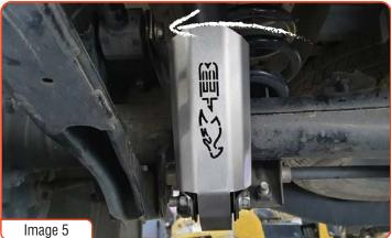
9. Remove the upper control arm bolt from the diff housing bracket and fit the shock absorber guard. Refit the upper control arm bolt Image 5 and fit 2x M14x80L bolt, 2x M14 nuts and 4x M14 washers to the two mounting holes that bolt the guard and the relocation to the diff housing.
