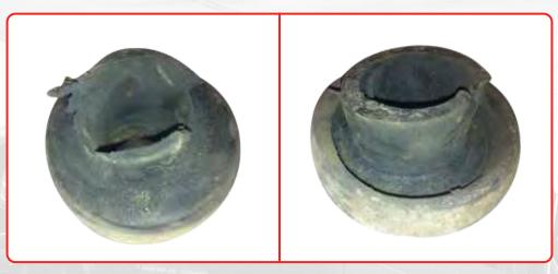
If your Patrol Radius Arm to Chassis Bushings are showing wear characteristics as illustrated in the pics opposite, it could be due to a number of reasons.
