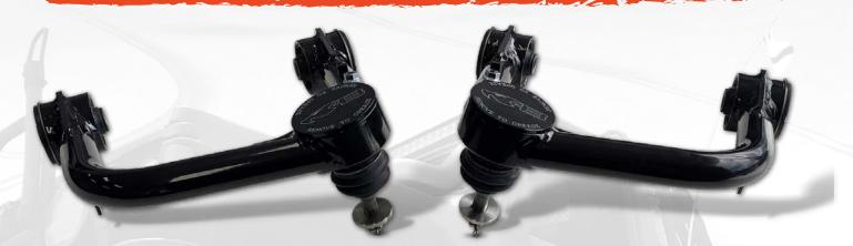
The Blackhawk4x4 UCA's are one of the best known brands on the market when it comes to fixing the steering kinematics with suspension lifts. The UCA4861T designed specifically to enhance wheel alignments with suspension lifts of 30-70mm on the 300" Land Cruiser are now available. The same standard features that can be found across the range are also included for the 300 series.
