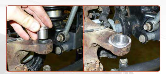
JK JEEPS have their Draglink in a low and vulnerable position on the passenger side knuckle, if wheeling in any rough terrain they run a very high risk of damage causing steering failure, or at best premature wear due to side impact of the rod/tie rod end.
