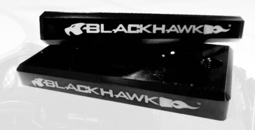
Prado 120 has a build variation with regard to front Sway Bar bracket hole spacing. There is no link back to VIN or year model, so measuring to ensure accurate ordering is required. The options available are 82mm or 76mm hole centre/centre. Sway bar relocation plates are now available for both options.
