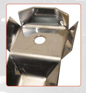
Manufactured from 2.0mm stainless steel, Roadsafe Multi-Fit Stone Guards are designed to bolt onto existing shock mounts using the existing shock bolt, protecting the shaft from stone pitting.
